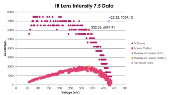
Graph 8: IV curve with infrared lens in front of light source for light intensity 7.5
