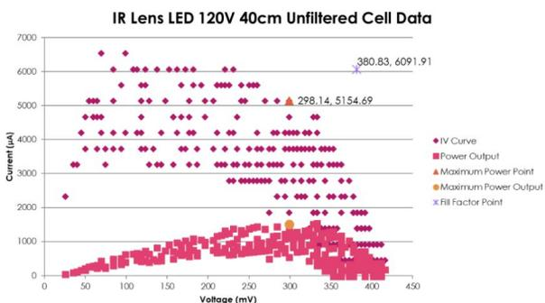
Graph 14: IV curve with infrared lens in front of LED light source at 120V
