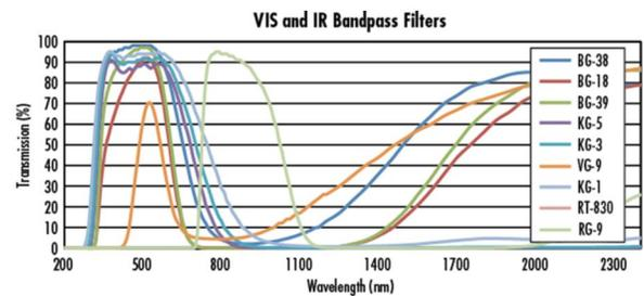
Figure 1: Graph showing optical filters effects after a light source passes through the filter
