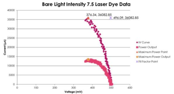
Graph 9: IV curve with thin film of laser dye for light intensity 7.5
