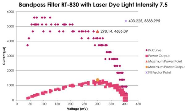
Graph 12: IV curve of Bandpass Optical Filter RT-830 with thin film of laser dye for light intensity 7.5
