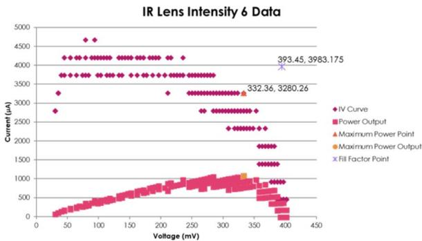
Graph 5: IV curve with infrared lens in front of light source for light intensity 6
