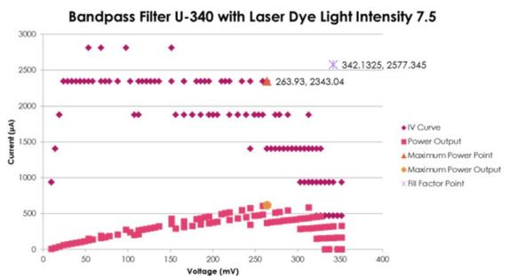
Graph 10: IV curve of Bandpass Optical Filter U-340 with thin film of laser dye for light intensity 7.5
