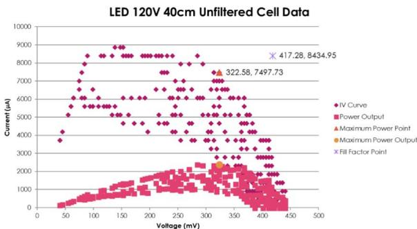
Graph 13: IV curve of control using a LED light source at 120V
