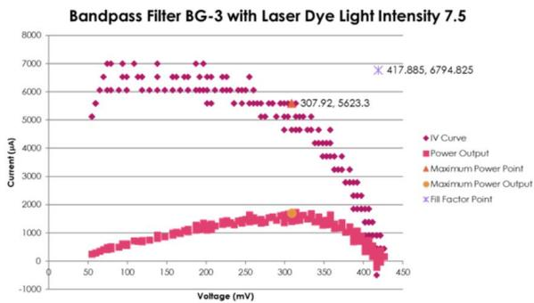
Graph 11: IV curve of Bandpass Optical Filter BG-3 with thin film of laser dye for light intensity 7.5
