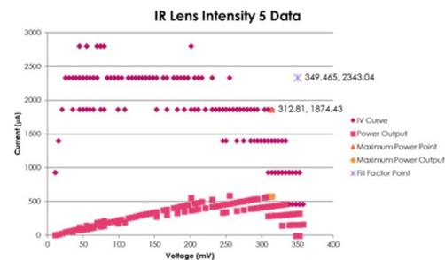
Graph 2: IV curve with infrared lens in front of light source for light intensity 5
