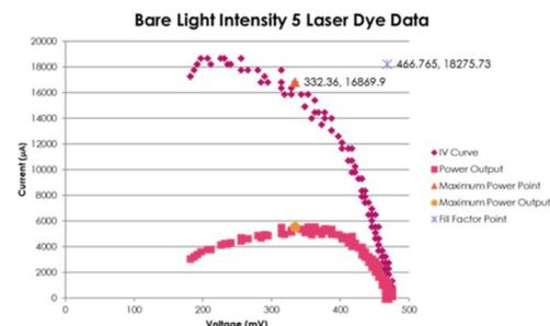
Graph 3: IV curve with thin film of laser dye for light intensity 5
