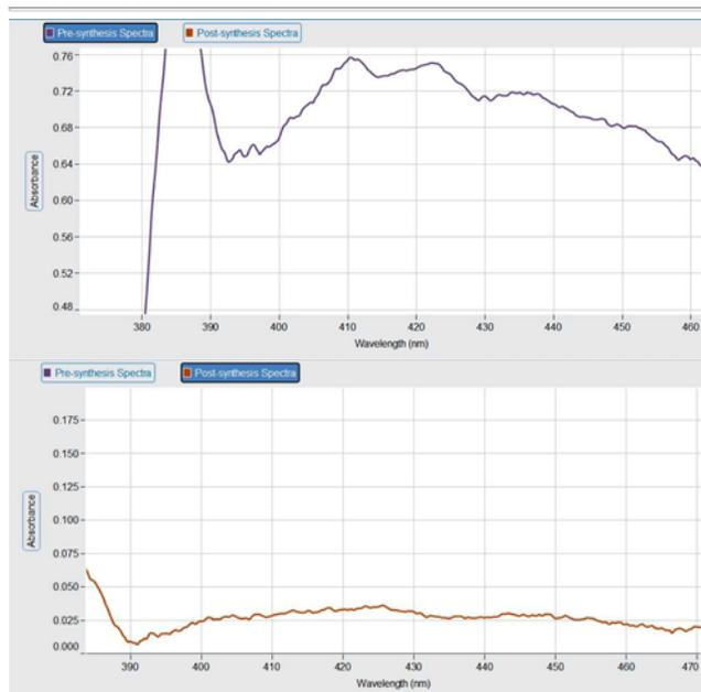
The comparison of the pre-synthesis solution (top) and the supernatant fluid after synthesis (bottom)
