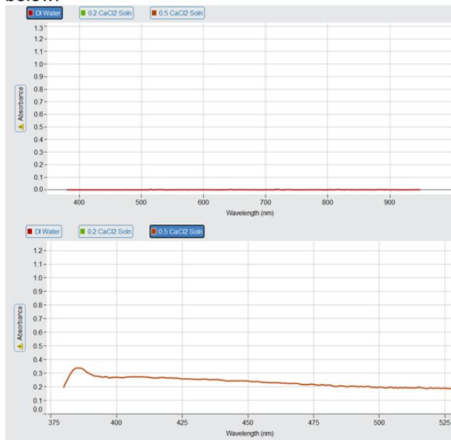
Comparison between the absorbance of the control (top) of DI water and the absorbance of one of the experimental groups (bottom) to test for the presence of nanoparticles.
