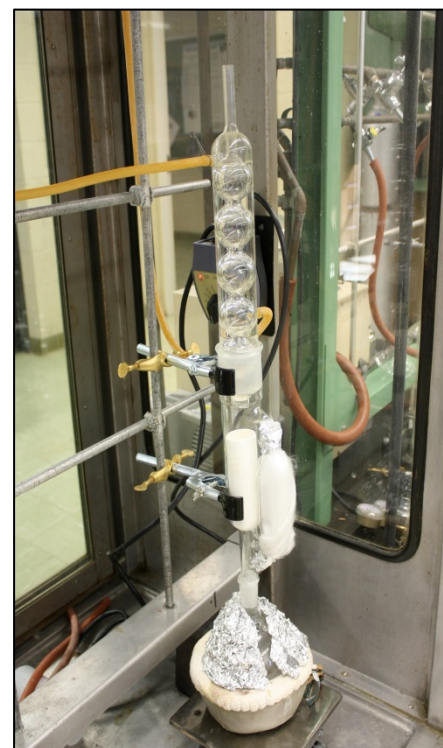
Fig 7. Soxhlet distillation apparatus for tea-infusion test
