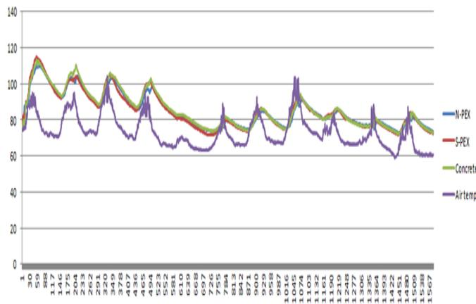
**Figure 3:** Uninsulated concrete slab curing temperatures as a function of time.
