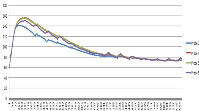
**Figure 4:** Insulated north wall curing temperatures as a function of time.
