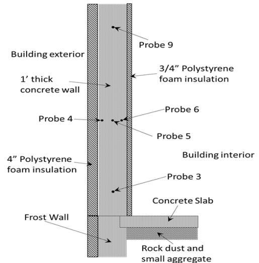
**Figure 2:** Cross section of the concrete wall, frost wall, and slab showing the locations of some of the temperature measuring probes.
