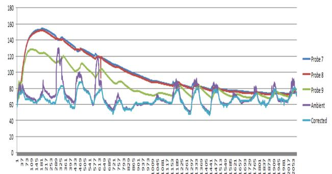
**Figure 5:** Insulated south wall curing temperatures as a function of time.
