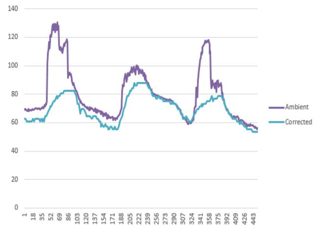
**Figure 6:** Expanded view of the ambient temperature as measured with a thermocouple close to the walls and floor, versus the temperature measured by the weather station at the nearby observatory.
