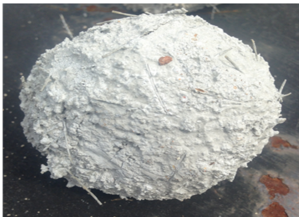
Figure 1: This is a picture of the TF Forming Systems' concrete mixture containing stainless steel helix fibers.
