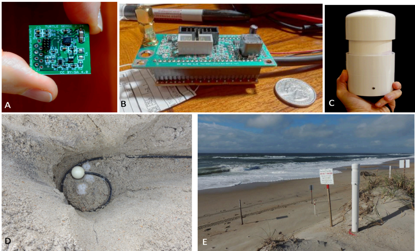
Figure 1. A schematic of the Turtle Sense system components (A) Sensor board (1" x 1") is sealed in a polyurethane ball designed to resemble a turtle egg. (B) Communications assembly is mounted in a 3" diameter PVC pipe (C) assembly (the quarter is for size reference). (D) The sensor ball is buried just above the sea turtle nest, with a buried cable leading to above ground communications assembly. (E) Turtle nest with functional Turtle Sense monitoring will remain in place until the hatchlings emerge and the nest is excavated by the NPS.
