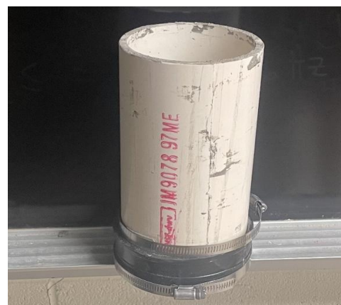
Figure 3: Concrete Mold, Where the drying phase occurs for 1-6 days
