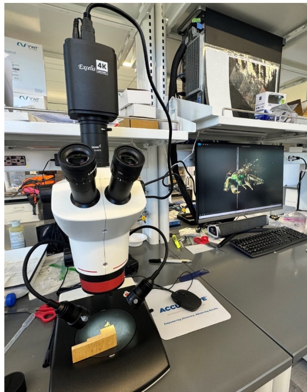
Figure 1. Microscope and camera setup for macro photography.
