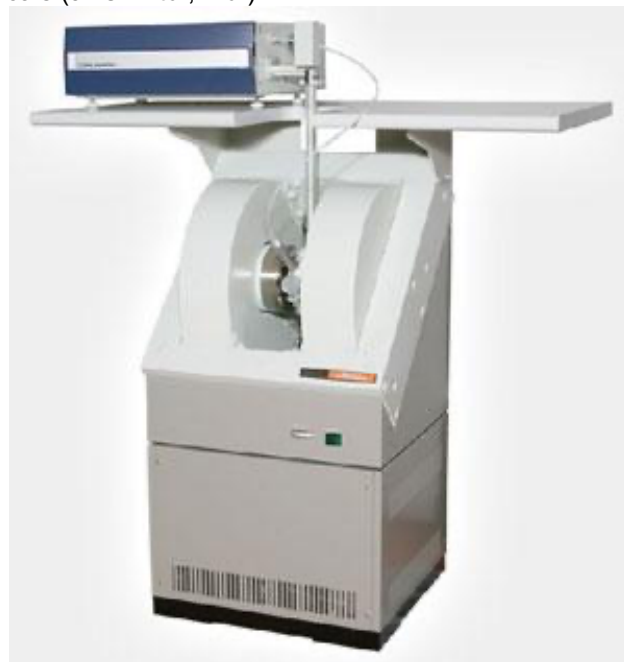
Figure 1: The JEOL X-310 ESR spectrometer detected electron spin resonance by measuring microwave absorption derivative signals under a magnetic field sweep. This spectrometer model was used in collecting ESR data for this research. (JEOL Ltd., n.d.).
