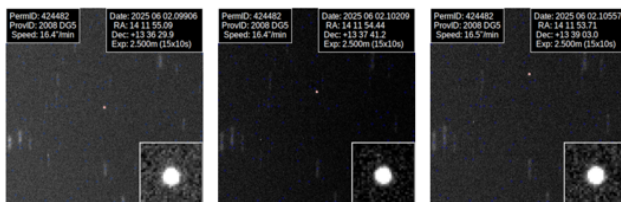
Figure 3. Example of completed observations taken from Tycho Tracker. Seen are three stacked images of 2008 DG5 with corresponding astrometric measurements. The target, 2008 DG5, appears as a bright point while background stars appear as faint smears.
