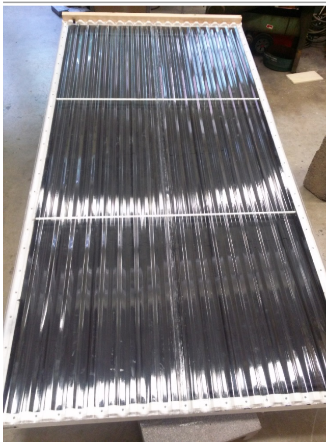
Figure 4: The solar collector after being applied silicon caulk
